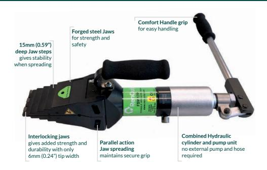
Max Spreading force: 163kN (16.3T)
