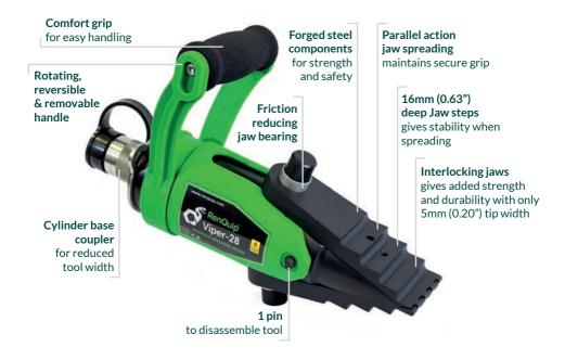
Max Spreading force: 277kN (27.7T)
