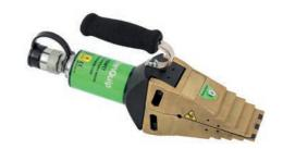
The contact areas between tool and flange are of a bronze material that is classified as nonsparking but the core material of the components remain as forged steel to maintain the strength and factor of safety of the tool.
